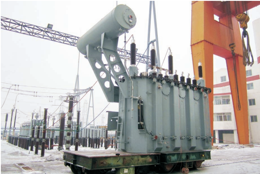
63MVA, 110kV Transformer under Short-circuit Test in Third-party Independent Test Lab
