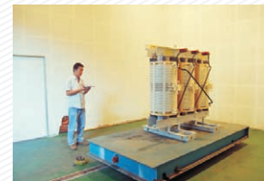
Test Chamber for Noise and Partial Discharge Measurement
